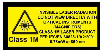
Additional laser safety information can be found on the Optek website. See application #221. Classification is not marked on the device due to space limitations. See package outline for centerline of optical radiance. Operating devices beyond maximum rating may cause devices to exceed rated classification
